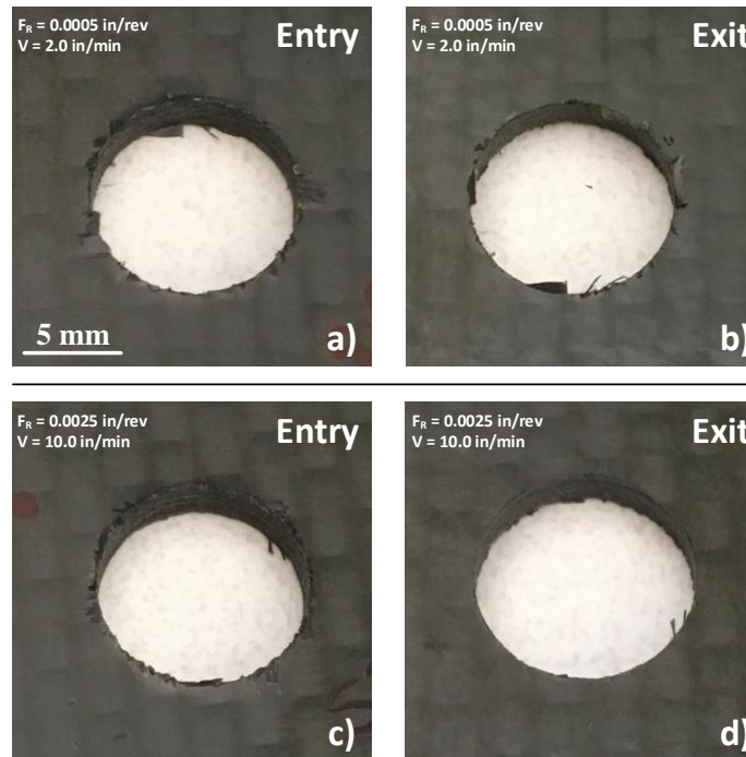
Figure 2-13: Surface imaging of CNC drilling for woven CFRP using a SPF drill ( N = 4,000 RPM): (a) and (b) entry and exit surfaces, respectively, for 4,000 RPM and 2.0 in/min; (c) and (d) entry and exit surfaces, respectively, for 4,000 RPM and 10.0 in/min.
