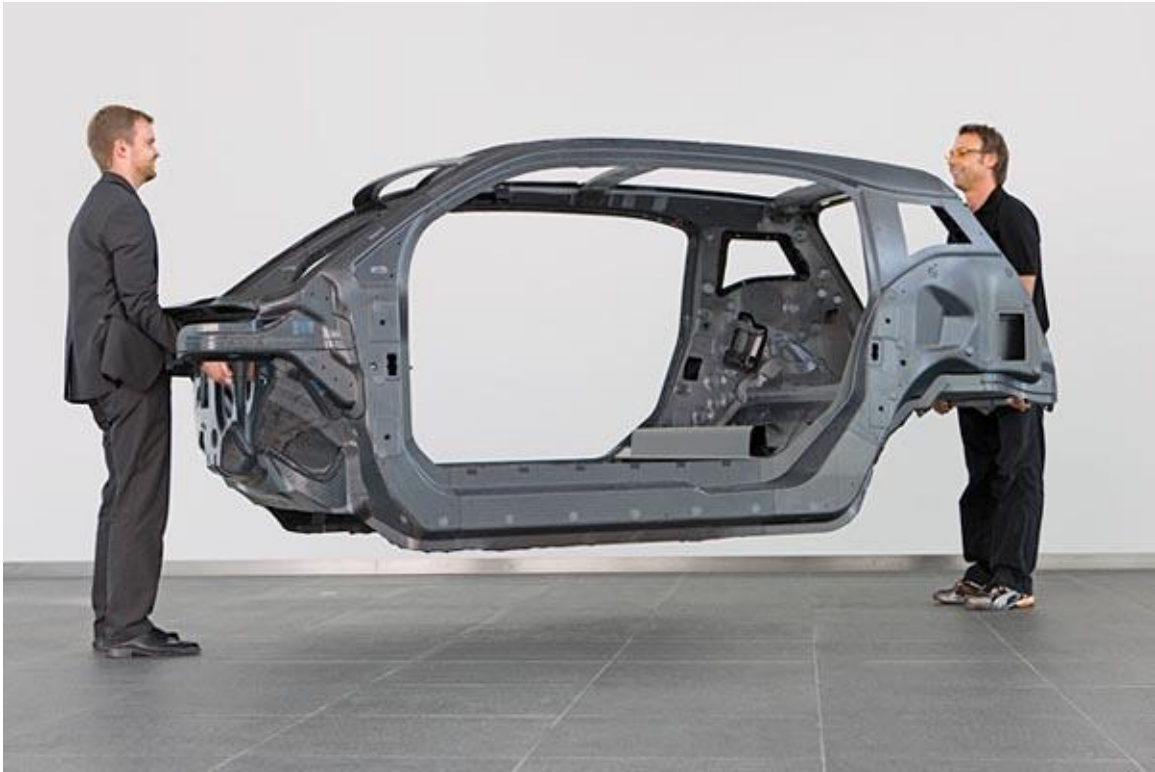
Figure 1-3: The “Life Module” of BMW’s i3 compact hybrid. Full carbon construction allows vehicle to achieve total curb weight of less than 3,000 lbs (EV World, 2013)
